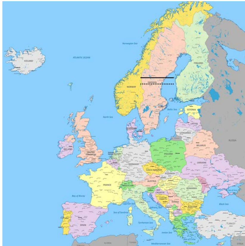
Figure 2: Europe according to the Mercator-projection. The solid line is the midpoint on the map, the dotted line is the midpoint as calculated using the details of the projection
